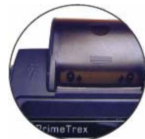
Full Graphic Thermal Printer, 22+ lines/sec
